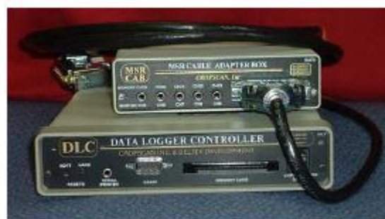
Figure D-2. Data logger controller &amp; cable adapter box.
