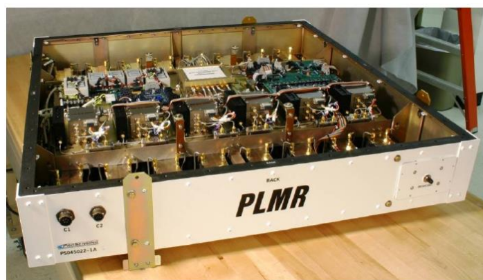
Figure 2-3. View of PLMR with the cover off.
