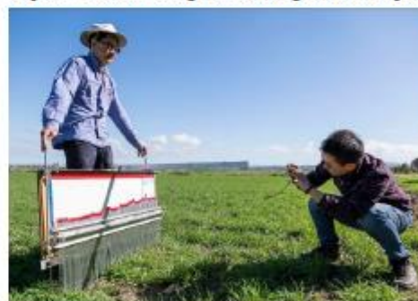
Fig. 4: Surface roughness sampling using a pin board profiler.
