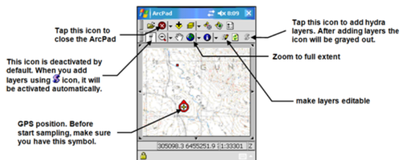
Figure 3. Customised toolbars for HDAS in ArcPad
