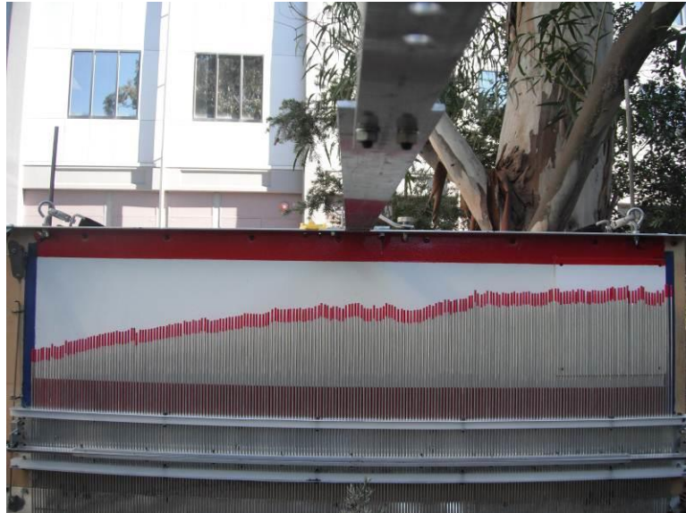
Figure 6-3. Pin profiler for surface roughness measurements.
