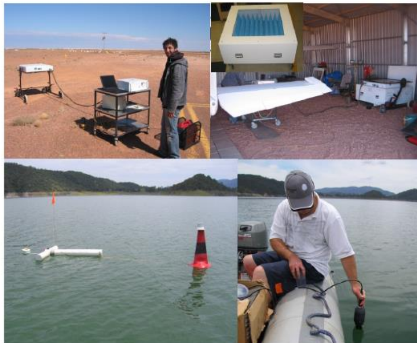
Figure 4-7. Upper left: undertaking a sky cold point calibration; upper right: undertaking a warm point calibration with the calibration box shown in the inset; lower left: the buoy used to monitor water temperature and salinity; lower right: undertaking a boat transect of water salinity and temperature.
